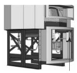
**3.** Attach the Controller to the mounting bracket of the Extension using the 1/4-20 bolts provided.
