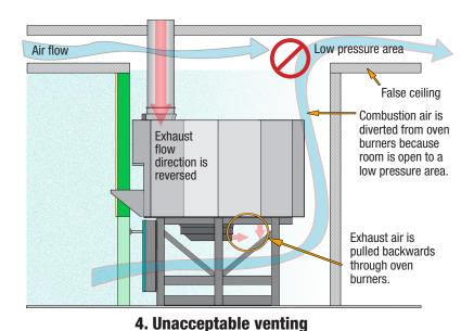
**Example 4** shows an incorrect installation where the enclosure surrounding the oven is open to the attic space above the ceiling. Air can move rapidly through the space enclosing the oven to the lower pressure area within the attic space. This can cause a downdraft situation at the oven, pulling air and heat backwards through the oven burners, leading to damage of oven components.
