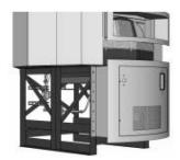
After the oven has been leveled, remove the Extension Panel Throttle Assembly which has been attached to the inside of the stand for shipping. Position the Lower Extension Assembly onto the front of the oven. It will rest on the guides that are welded to the oven legs. Attach the assembly to the oven legs using the supplied 1/4-20 nuts, bolts and washers.
