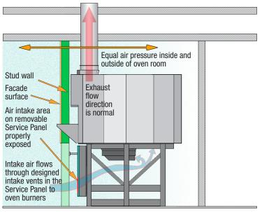
**Example 1** shows a proper installation. The enclosure around the oven is completely sealed so that the only air entering the space beneath the oven comes through the oven Service Panel.
