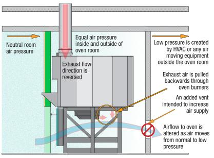
**Example 3** shows an incorrect installation where an additional vent was added to the wall behind the oven, creating an air pressure difference causing air movement beneath the oven and disrupting the operation of the oven burners. This air movement can be so severe as to cause a downdraft, pulling the exhaust down the oven flue and backwards through the burners, leading to heat damage of oven components.
