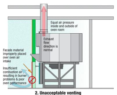
**Example 2** is not acceptable because the combustion air intake is blocked, preventing combustion air from reaching the oven burners. The burners will not function properly, and will lead to damage of oven components.
