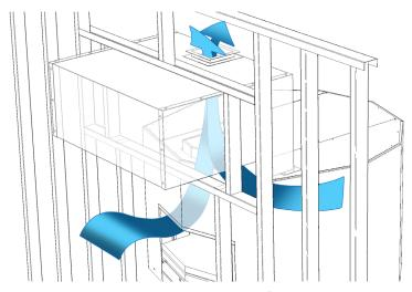
**Incorrect installation.** No flashing has been installed so air being pulled up the sides of the oven from beneath.
